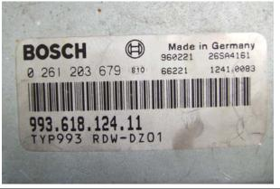
Turn the ECU upside down & you will see 10 small metal tabs. These tabs need to be bent up to allow the cover to be removed. Use a small screwdriver or similar to start with and then pliers. When the tabs are bent vertical it should be possible to remove the metal cover.
