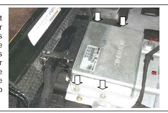
The label on this ECU displays the Bosch **0 261 203 679** part number that we require. It will also help to supply the **993.618....** number.
