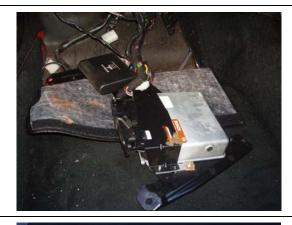
The picture on the right shows the ECU (removed for illustration purposes) so you can see the number from this ECU that reads 0261 200 195 & this is all we need. It also helps to confirm your vehicle year & model when ordering.
