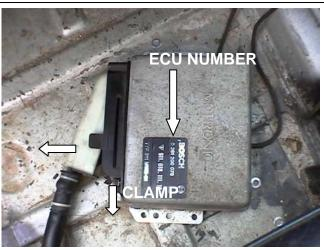
Turn the ECU upside down & you will see 10 small metal tabs. These tabs need to be bent up to allow the cover to be removed. Use a small screwdriver or similar to start with and then pliers.
