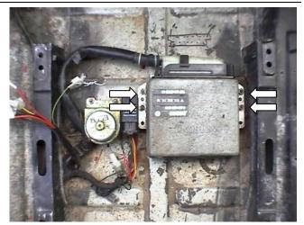
Lift the ECU forward & remove the connector plug by pulling the metal clamp.
